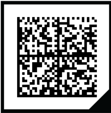
Figure 3 – Example of a 2D data carrier for the Material Digital Passport, embedding the Identification Code https://www.domain-abc.com/4167555e-8ee3-11ee-b9d1-0242ac120002 4167555e-8ee3-11ee-b9d1-0242ac120002 is a hexadecimal UUID generated as per ISO/IEC 9834-8:2014.
